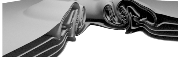
Fig. 18. Centerline slices through vortex sheet (left) and vorticity (right) for five-layer interface with \Sigma\theta^* = 1 ; \delta^* = 0.2 , rendering is at t^* = 8 .
